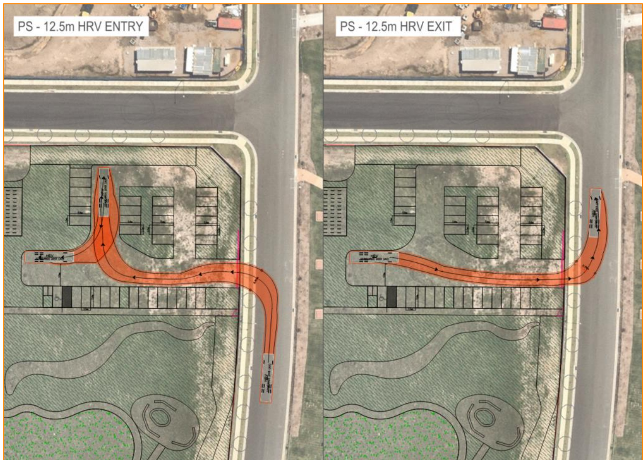
Figure 6: Service Vehicle Access for 12.5m Heavy Rigid Vehicle (HRV)
